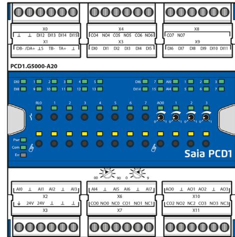
The E-Line RIO modules are controlled via RS-485 and enable decentralised automation using industrial quality components. The data point mix is specifically designed for applications in the HVAC sector.
