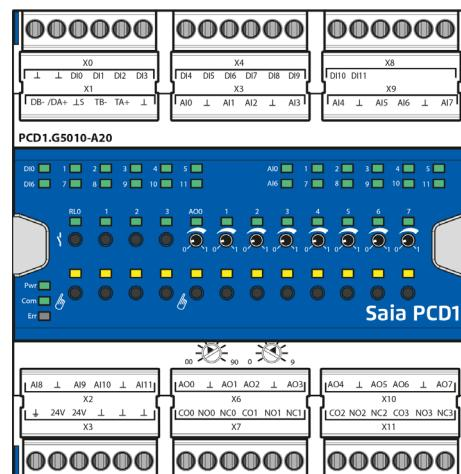
The E-Line RIO modules are controlled via RS-485 and enable decentralised automation using industrial quality components. The data point mix is specifically designed for applications in the HVAC sector.
