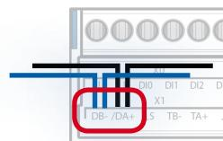
Flexible RS-485 cables with a cross section of no more than 0.75 mm<sup>2</sup> must be used for bus wiring. A cable cross section of 1.5 mm<sup>2</sup> is allowed per terminal.
