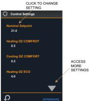
The TRC-P devices are configured to operate in different modes via the configuration parameters accessible through the maintenance mode.
